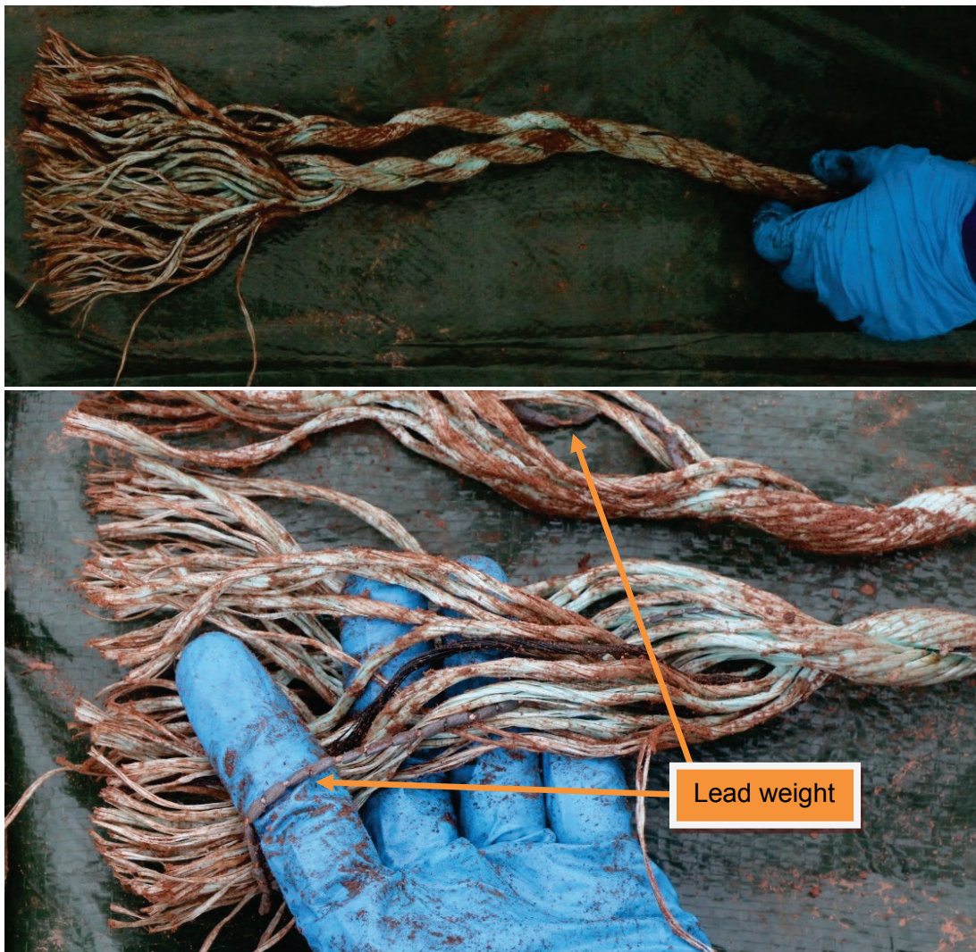
Figure 14. Cut, slightly frayed bitter end of Segment 2 with lead weight visible.
